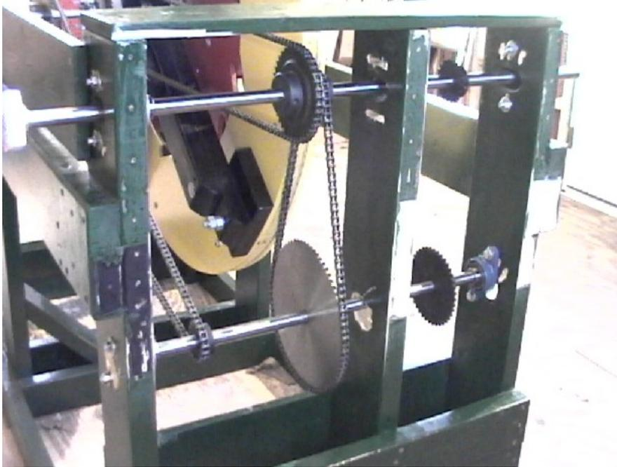
Preston Stroud Toy Test Model for evaluating concepts of gear ratio and weight patterns on the BuzzSaw Gravity Wheel
