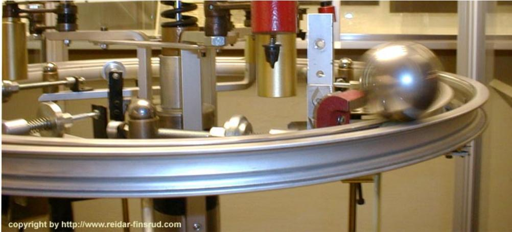
The steel ball continually runs around the path formed by the 2 concentric circular aluminum tracks. The ball is about 2.7 inches in diameter and the track has a diameter of about 25 inches. You can see one of the 3 horseshoe magnets next to the ball in the 3rd pic.
